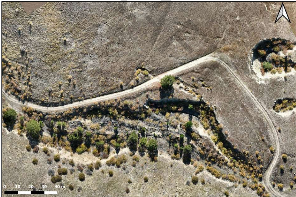
Figure 17. Aerial photograph showing main workings, access road disturbance, eastern sluiced areas, and potential race features.
