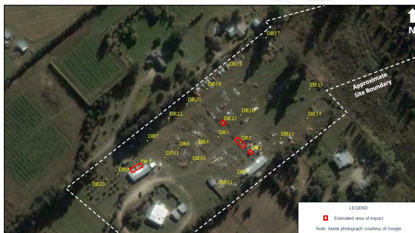
Figure 8. Excerpt of the Insight Engineering site plan, red squares identify the areas to be remediated.
