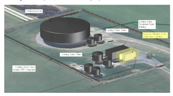
The diagram above shows the location of the newly designed filtration and ultraviolet disinfection container portrayed on the current Ranfurly water treatment plant site.
