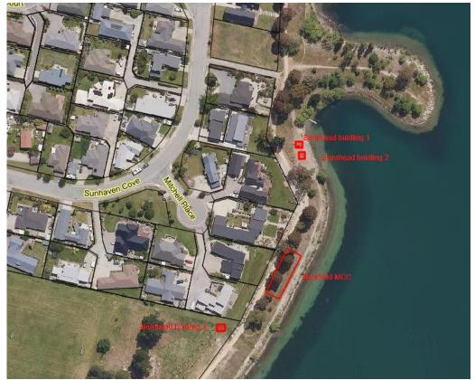
Figure 5: Plan view of the proposed locations of the borefield electrical switchboard and Motor Control Centre building (MCC building) and the borehead buildings
