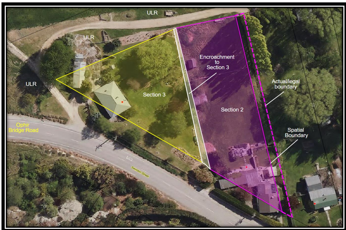
Figure 4 – Plan of private encroachment and approximate location of true eastern boundary of Section 2.
