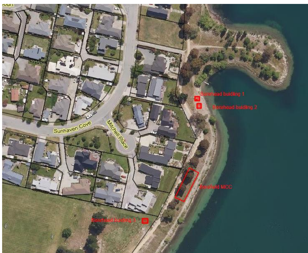
Figure 5: Plan view of the proposed locations of the borefield electrical switchboard and Motor Control Centre building (MCC building) and the borehead buildings
