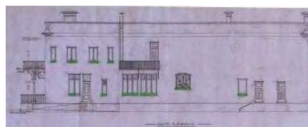
Fig. 262 Highlighted areas of expressed brick elements on the south elevation as detailed by Anscombe on the original plans.
