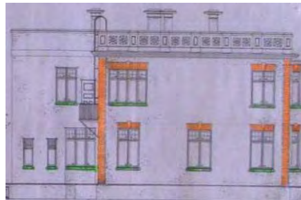
Fig. 264 Highlighted areas of expressed brick elements on the east elevation as detailed by Anscombe on the original plans.
