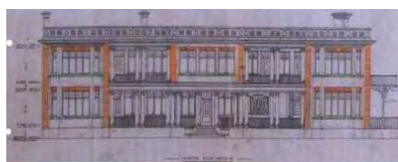
Fig. 261 Highlighted areas of expressed brick elements on the north elevation as detailed by Anscombe on the original plans.
