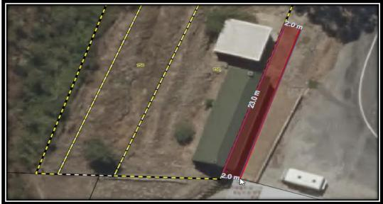
Figure 9 – Plan of less expensive option for legalising the encroachment.
