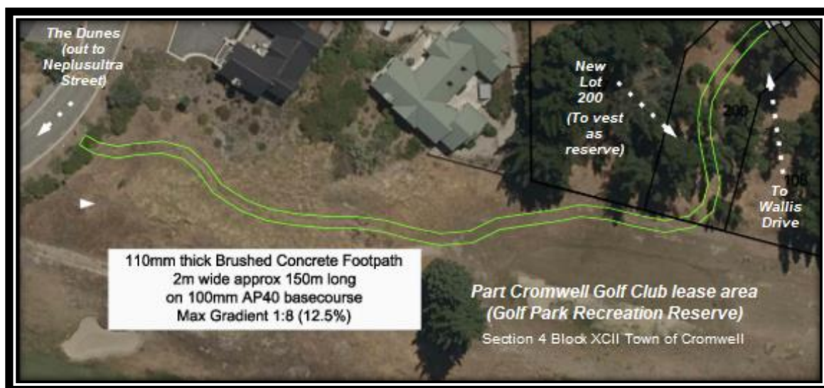
Figure 2 – Construction details and map of path overlaid into GIS.
