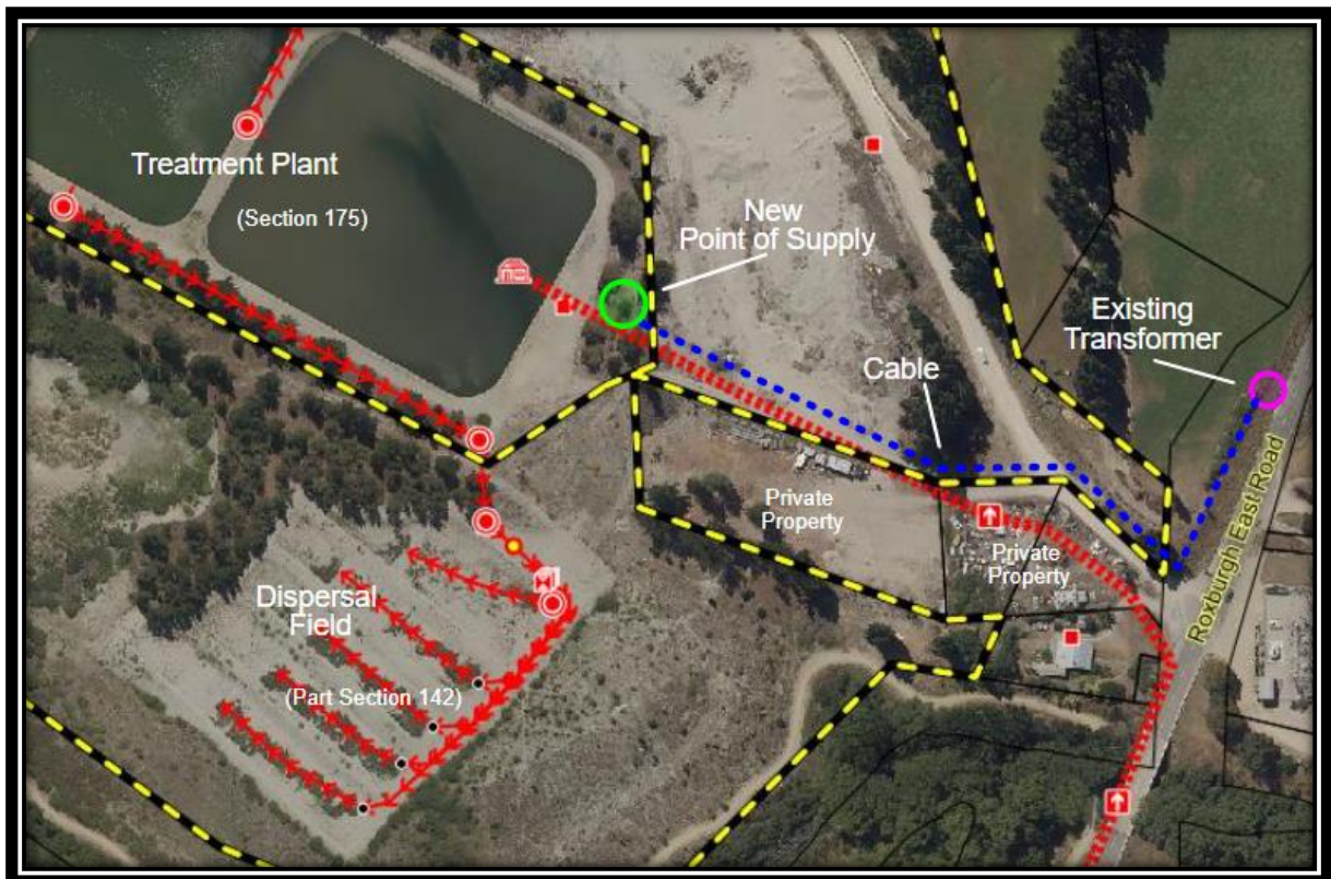
Figure 2 – Proposed cable, existing transformer, new point of supply, and the existing wastewater infrastructure
